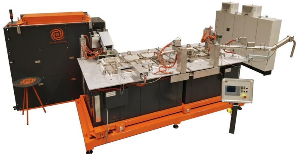
Modern two-furnace magnesium melting system including dosing system and cast-on return.
