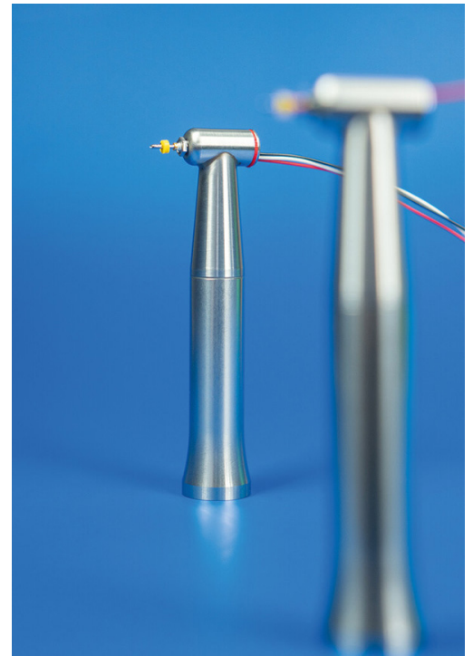
Endodontic handpiece Image: Fraunhofer IKTS
