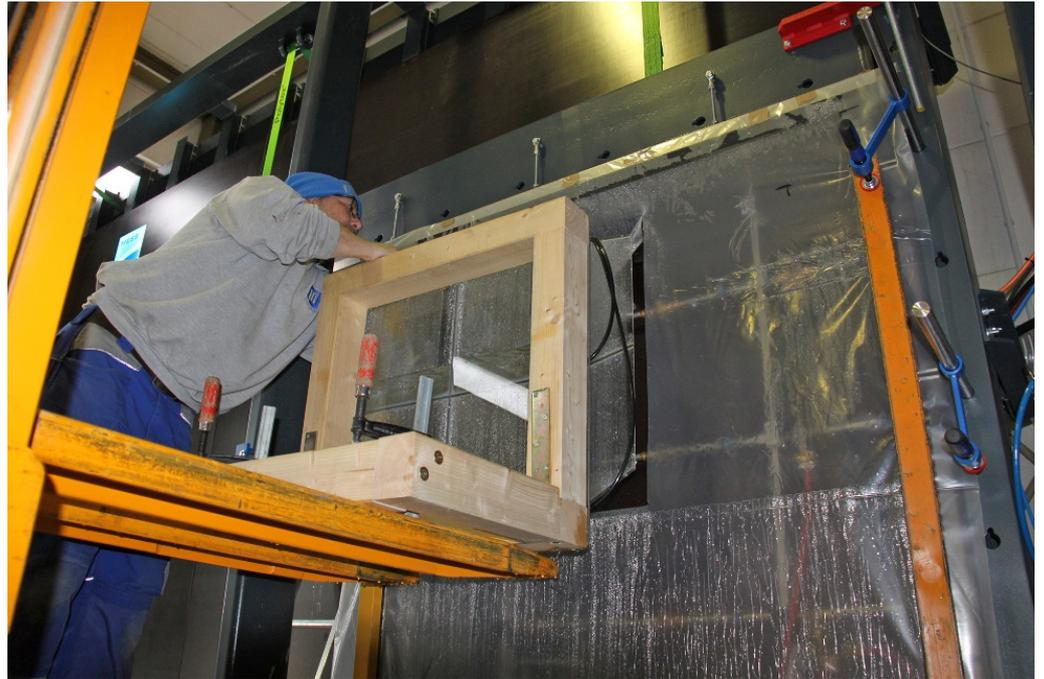
*The calibration of the water spray system according to ASTM E 331 with the help of the so-called Catch-Boxes is important before testing the watertightness according to NAFS (North American Fenestration Standard).*
