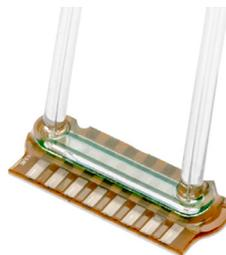
*Continuous multiparametric biosensor with a measurement volume of only 1 µl to be fed by body fluids from micro dialysis*
