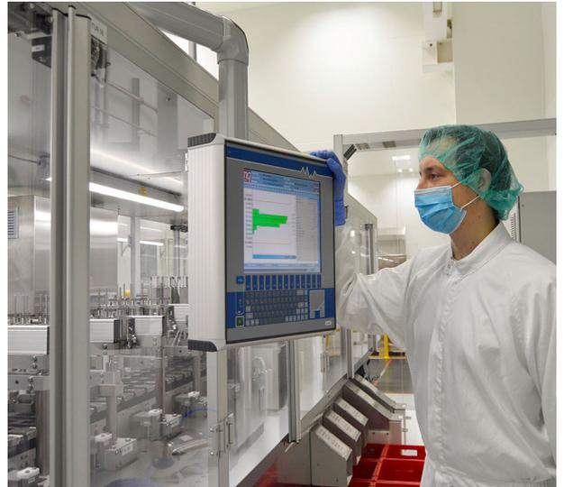
Project planning and development of automated production systems with high quality requirements round off the repertoire for specific customer solutions. On a total of 26 fully automated assembly lines the plastic components are assembled in the clean room in accordance with the assembly concept to form subassemblies and, if required, individually finished and packaged.
