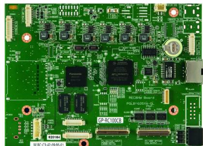
The GP-RC100 provides the opportunity to record the live picture directly to a USB device or access them from a PC via IP network. Ease of operation for this recording solution is provided through a direct connection to the Panasonic OEM micro camera solutions GP-US932, GP-KH232 & GP-UH532CB (enables 2K recording only).
