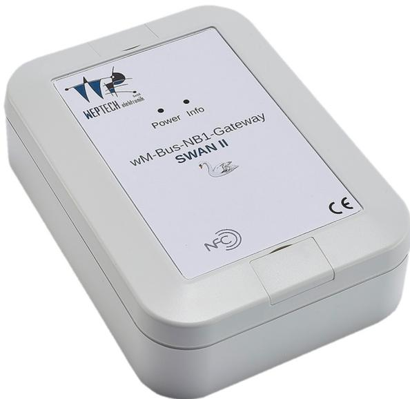
The battery operated gateway SWAN 2 directly links wireless M-Bus devices to the cellular network using the new LTE Cat NB1 technology and optionally supports the wired interfaces L-Bus, RS-485 or 2x Pulse. The OMS compliant wireless M-Bus interface supports mode S, T and C with frame format A and B.
