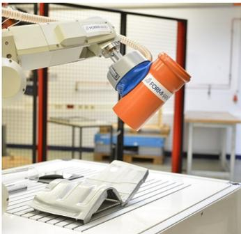
One gripper, various parts. The FORMHAND grippers automatically adapt to the objects.
