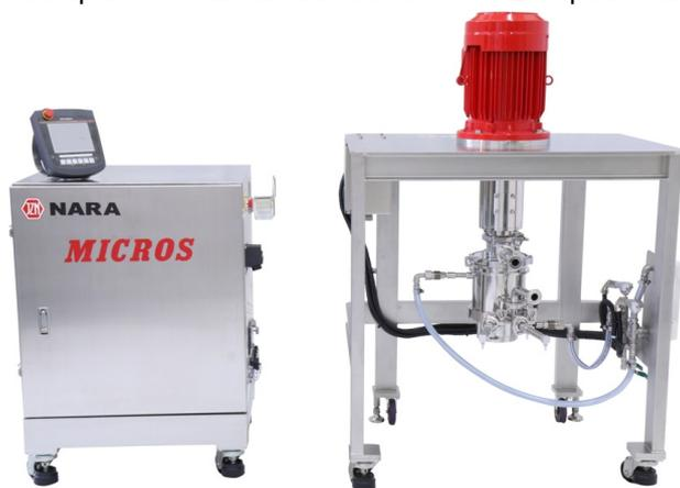
Compared to a conventional ball mill, Micros is a wet milling machine with a completely different milling mechanism. The compression and shear force applied to the materials are generated by the movement of the milling rings against the lining of the vessel.
