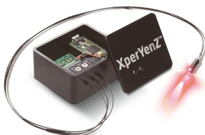
The fiber optic sensor from trinamiX combines for the first-time, the properties of classic fiber sensors with precise, absolute distance measurement. Until now, fiber optic sensors were only able to detect the presence of objects. The novel fiber optic sensor measures distances, precisely, robust, and fast – even in challenging environments.
