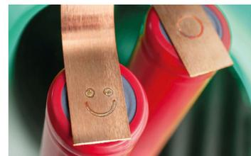
*In battery technology, lasers already enable extremely precise and stable connections today: Laser bonding can be used, for example, to weld copper ribbons onto battery cells.*
