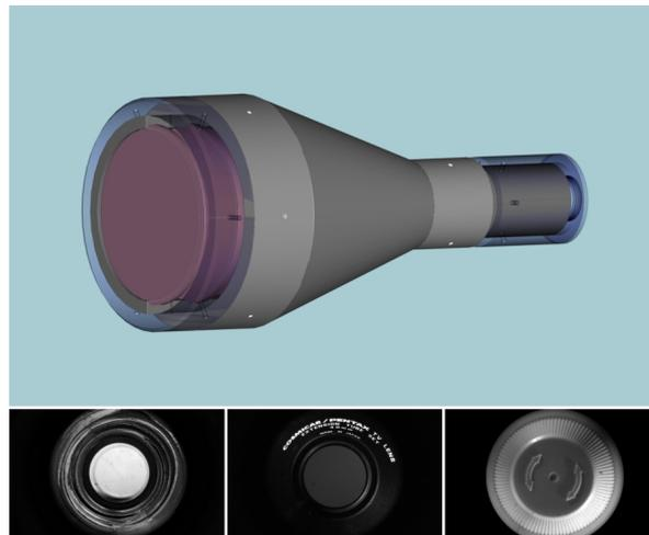
This is made possible by a special optical construction which uses an entrance pupil being a real image of the aperture stop. Lenses of this type are extremely rare on the market. Eureca develops such optical systems tailored to the customer's needs. The new pericentric lens covers object diameters of up to approximately 40 millimeters and is suitable e.g. for the inspection of threads of bottles, caps and other objects which are preferably of cylindrical shape.
