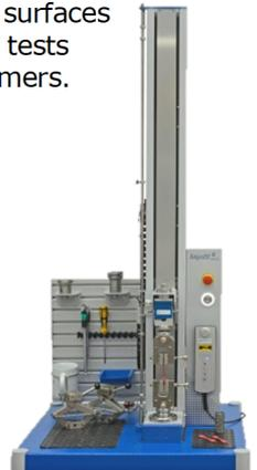
In the Inspekt duo, this constructive approach is implemented on a two-spindle testing machine. The big brother is designed for test loads between 5 and 30kN.
