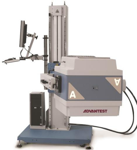
Because of its high integration and decentralized resources, the Advantest V93000 SoC series offers unprecedented scalability. Its modular design makes it easy to extend the system with new modules and instrumentation, as test needs change or evolve.
