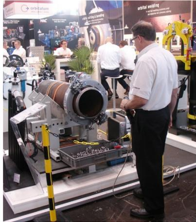
Robots are generally very widespread in welding, but not particularly in TIG welding. TIG is used "almost never in conjunction with narrow gap welding or the welding of pipe-floor joints." This is due to legal requirements which include, for instance, a shielded zone without user access – unlike conventional automation solutions. Polysoude, however, allows the use of robots in TIG welding.
