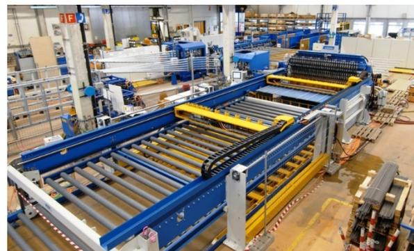
This can only be done by using the optimised high efficiency MG316 mesh welding machine and the newly developed highly flexible but high performance MG800 mesh welding machine. This combination allows flexible production development and, nevertheless, low processing costs.
