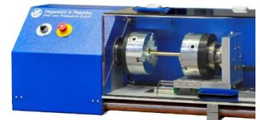
The torsion tester is used in science, research and teaching, in testing laboratories and in production control during production.
