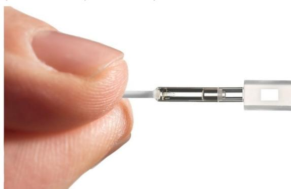
This is possible by measuring the optical refractive index with a miniaturized optical interferometer of 2mm size. No mechanical resonances are limiting the bandwidth of the sensor and a frequency range of 10 Hz – 1 MHz is accessible, exceeding the bandwidth of conventional acoustic sensors by a factor of ten.
