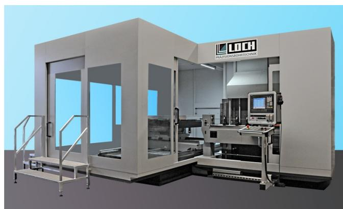
The changing of tools at the milling spindle is carried out power-operated manual or in connection with a tool changing system, which can be offered optionally. The Deep Hole Drilling Unit is completely covered and matches the Safety Guidelines of the CE-Standards, as well as the operational safety prescriptions.
