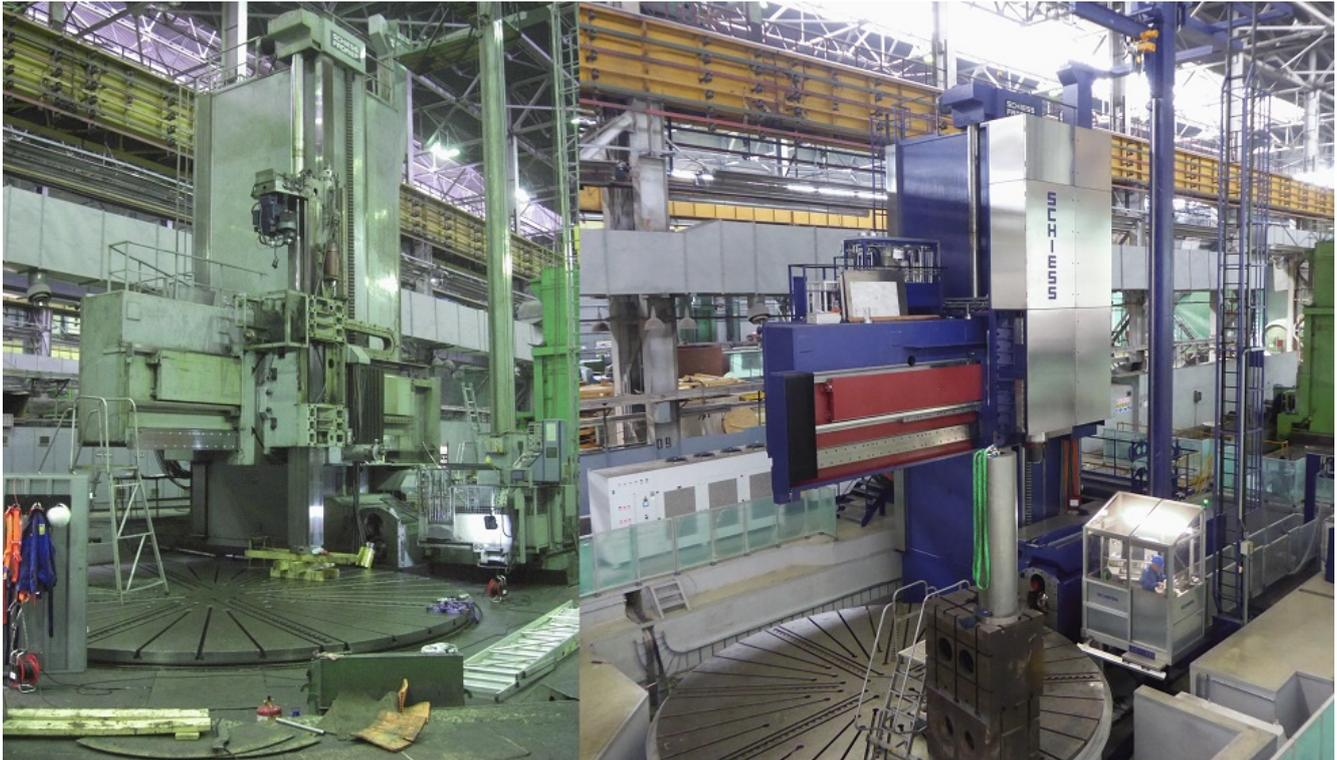
*By having the machine retrofitted, the customer saves receives a nearly-new machine at a lower cost. Furthermore, this machine suits the existing layout and fulfills all current technical requirements.*
