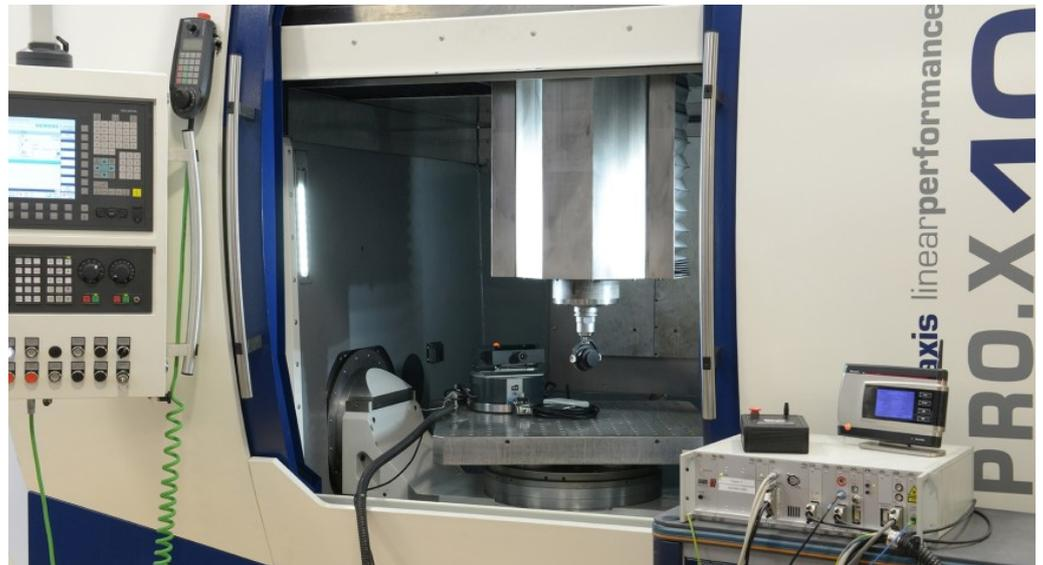
The Fraunhofer IPT examines how a machine component for vertical movements (Z-axis) made of carbon-fibre composites behaves in a machine tool and how the Z-slide can be optimised
