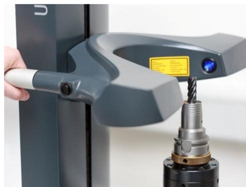
A sensor controller integrated into the handle activates the laser in the measuring arm when touched. The laser simplifies quick movement to the desired tool position, as the current camera position is always visible as a red light dot. Fixed tools, in particular, such as solid carbide or PCD tools, can be quickly and easily measured and set using the UNISSET-C. The maximum tool diameter is 400 mm, the maximum tool length also 400 mm.
