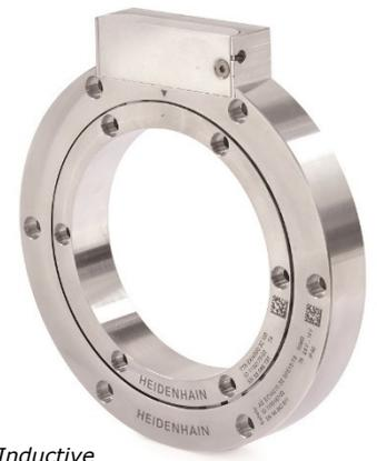
**Inductive hollow-shaft rotary encoders ECI 4000 and EBI 4000 from HEIDENHAIN for direct mounting, with a hollow shaft diameter of 90 mm**
