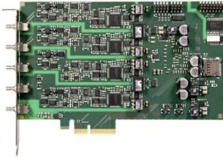
4 analog inputs, 4 current sources for the connection of ICPTM sensors
