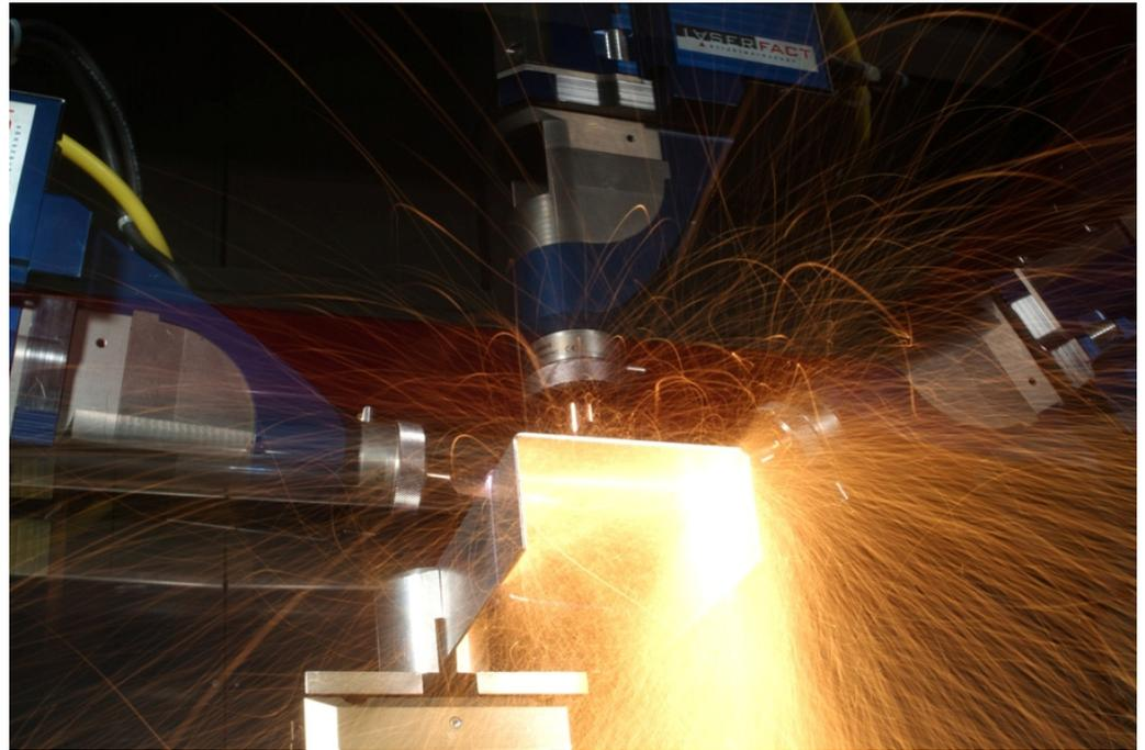
*Laser combi-head for cutting and joining as well as additive manufacturing by means of laser metal deposition.*
