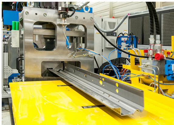
With this in mind Dreistern has developed the Multifunctional Rollforming System. The idea was to evolve a tube mill and a rollforming machine into a sheet metal machining system. Companies can now supply not only tubes but also have the ability to produce all products combining rollforming, punching, bending and welding that will positively contribute to their bottom line.
