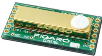
High precision NDIR-CO<sub>2</sub>-sensor module facilitates measuring the indoor air quality
